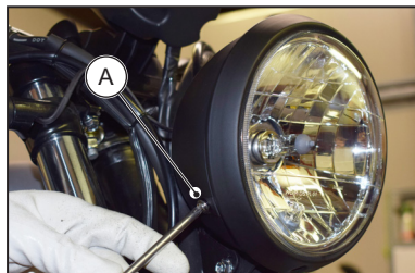
A. Fixing screws of the headlight group
