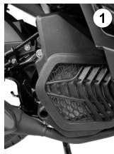
1. There is a radiator tank at the bottom of the right rear pedal.
