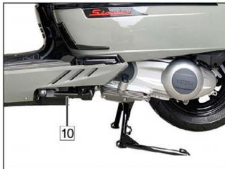
7. Side (10) switch at horizontal position.
