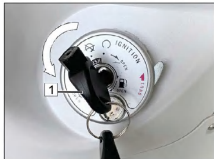
1. With the key(1) in the "OFF" position, turn it counterclockwise to open the seat(2).
