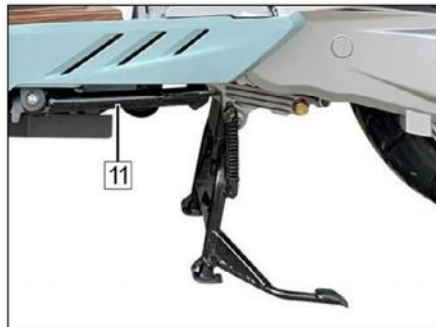
7. Side (11) switch at horizontal position.
